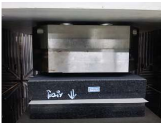
(a) Uniform pressing testing experiment using the surface plate
