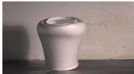
**Fig. 6.** Change due to heating of the polystyrene cup.
