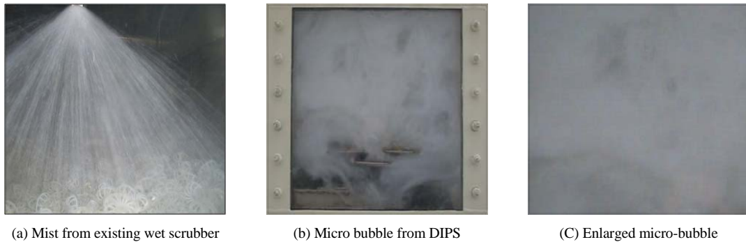
Fig. 3. Comparison of mist and micro bubble: (a)Mist from existing wet scrubber (b)Micro bubble from DIPS (c)Enlarged micro-bubble.
