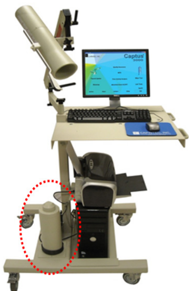
Figure 1 NaI(Tl) well type counter; Captus 3000, Capintec, U.S.A was used for this study
