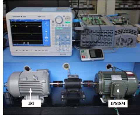
Fig. 12. Experimental platform of 2.2kW IPMSM.
