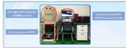
Fig. 2. High Purity Germanium (HPGe) Gamma-ray spectroscopy system.
