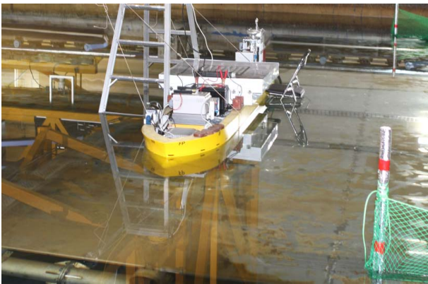
Fig. 1 KVLCC2 model ship on the false-bottom
