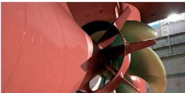
Fig. 1 Mewis duct of form of stator protruding through duct
