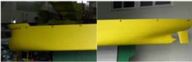
Fig. 14 Model ship of 176k bulk carrier
