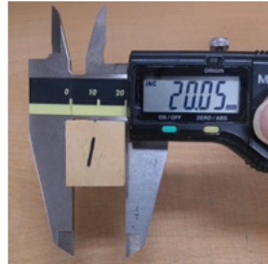
Fig. 6. Measurement of length with vernier calliper.
