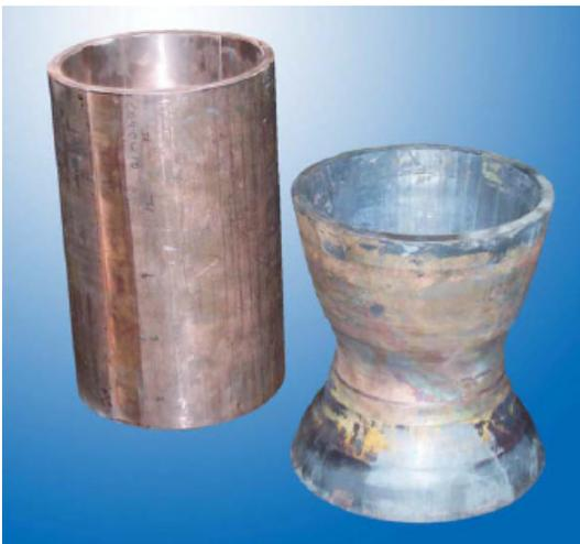
Fig. 10 GRCop-84 nozzle throat before and after spinning[10].
