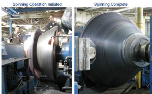
Fig. 13 Spinning operation(left) and nozzle liner after spinning(right)[12].
