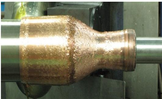
Fig. 7 Spinning product of nozzle throat part of small-scale thrust chamber by KARI[9].
