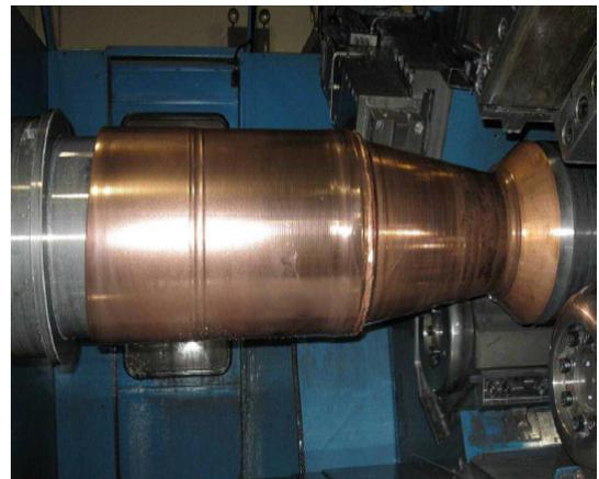
Fig. 11 Flow forming of chamber for LE-X engine [12].
