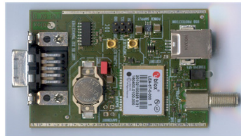
Figure 2. EVK LEA 6T receiver and antenna
