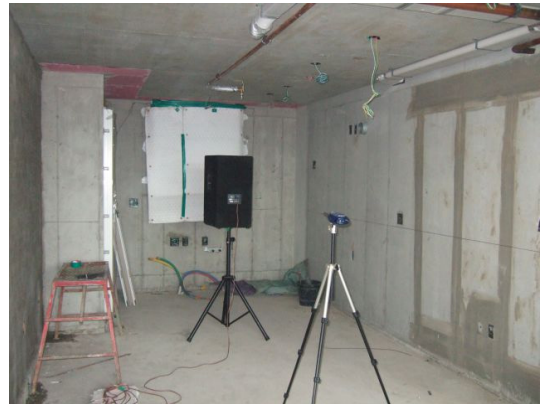
Fig. 9 Site insertion loss test of temporal barrier for gang form demolition work (white noise)
