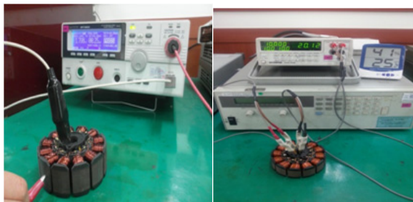
[Figure 3] Dielectric test and Resistance measurement
