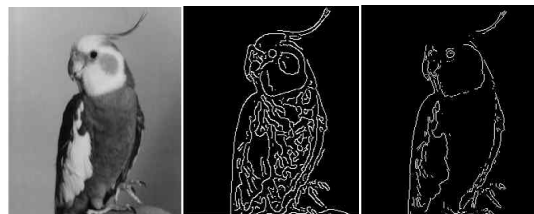
(Figure 1) Gray image(left), Canny operator(mid), Edge of FIS(right)
