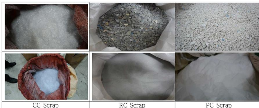
**Fig. 1.** Post-consumer PVC scrap used in this study.
