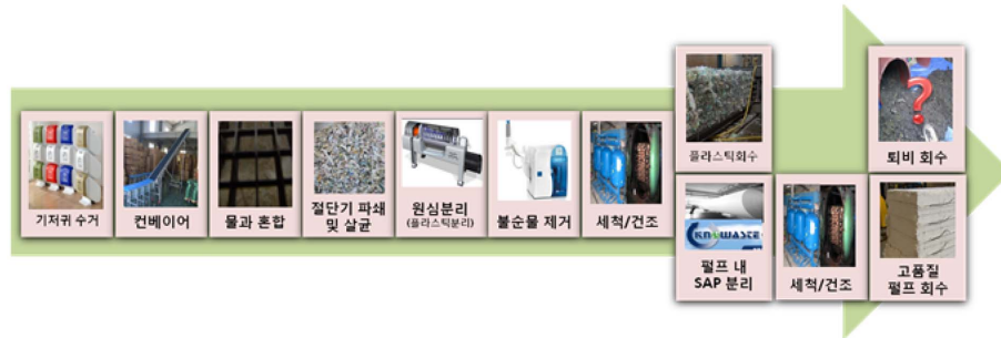
Fig. 1. Diaper recycling process by Knowaste.
