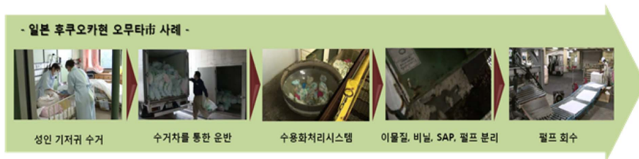
Fig. 2. Diaper recycling process by Totalcare in Japan.
