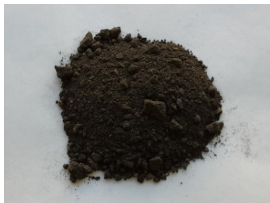
(b) Food wastewater treatment facility carbide
