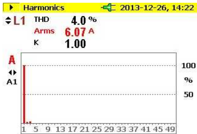
Fig. 22. Total harmonic distortion (THD) of input current at 320V DC reference voltage.
