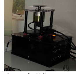
Fig. 10. Experimental setup for DC motor speed control.
