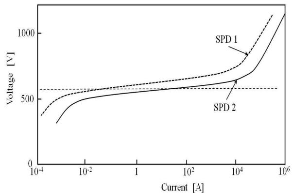
Fig. 2.  $V-I$  characteristic curves for two metal oxide varistors
