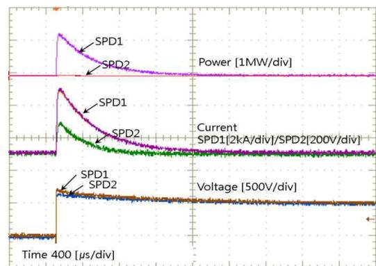
Fig. 4. Typical waveforms of the residual voltages and currents of each SPD in Case 1
