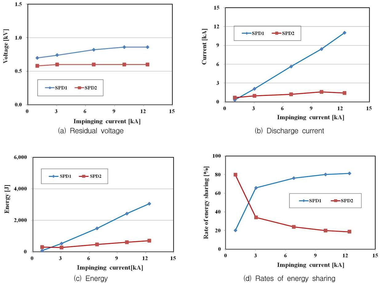
Fig. 9. Measured results of the residual voltages, discharge currents, energy, and sharing rates of each SPD as a function of the impinging current in Case 3
