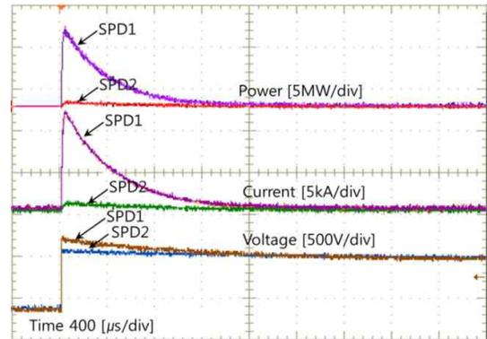
Fig. 6. Typical waveforms of the residual voltages and currents of each SPD in Case 2
