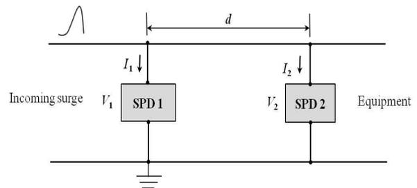
Fig. 1. Cascaded configuration of two parallel connected metal oxide varistors
