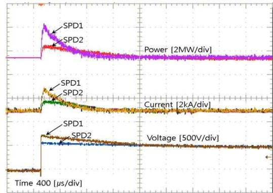
Fig. 8. Typical waveforms of the residual voltages and currents of each SPD in Case 3
