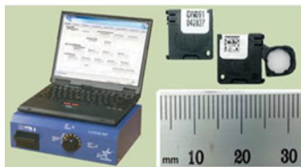
Fig. 1. Optically stimulated luminescence dosimeter and reading system.
