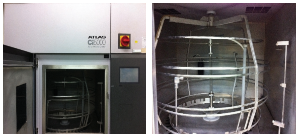
Figure 1. Weather resistance test(Xenon Arc Weather-Ometer Ci5000).
