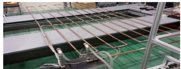
Figure 6: External appearance of pipe & thermocouple
