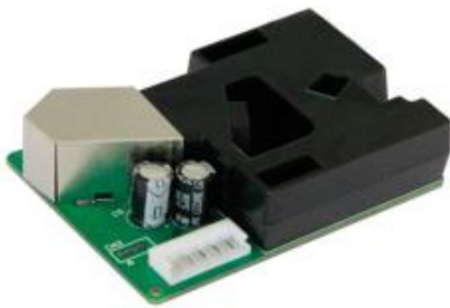
Fig. 4. Dust sensor installed in TREMS
