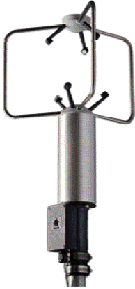
Fig. 3. Ultrasonic anemometer installed in TREMS
