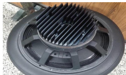
Fig. 2. Real picture of the woofer device with the developed heat sink
