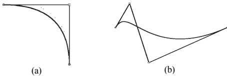
Fig. 7. Comparison the number of control points (a)Single curvature (b)Multiple curvature
