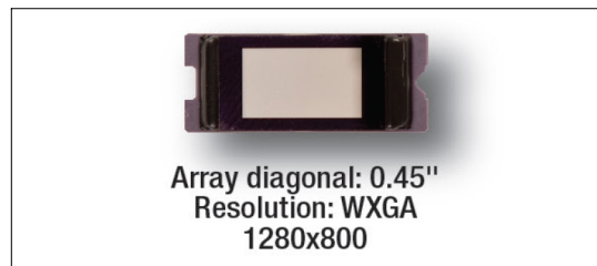
Fig. 3. Applied DMD(DPL4500) in This Paper (Texas Instruments)
