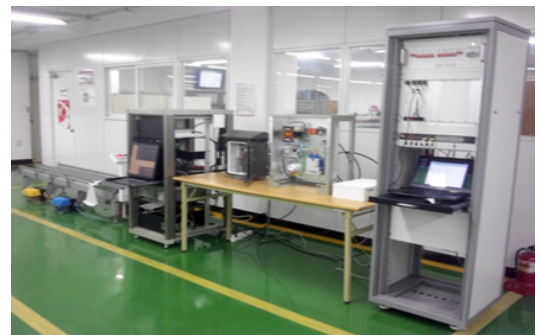
Fig. 18. Test Bed for Axle Counter test
