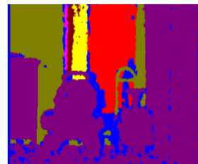
(b) Depth image obtained with depth-pixel processing; purple indicates the distances of toy vehicle 1 and toy vehicle 2
