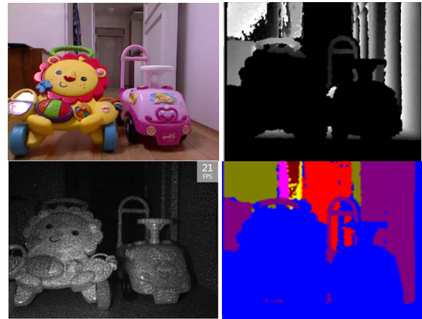
Fig. 2. Different types of image that can be captured with a Kinect sensor: RGB images, depth images, infrared images, and color-depth images.
