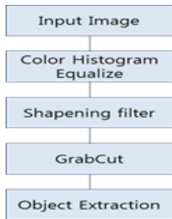
[Fig. 3] A Flow Chart of proposed method
