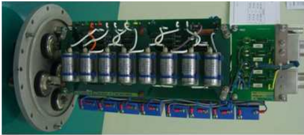
Fig. 4 The Inside of traction inverter
