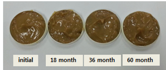
Fig. 10 MOV long life lubricant
