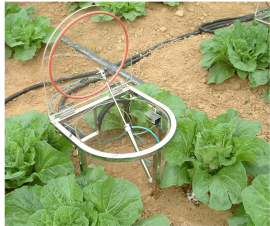
Fig. 1. Steady-state chamber for collecting N 2 O in soil.
