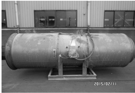
(a) High pressure jet fan
