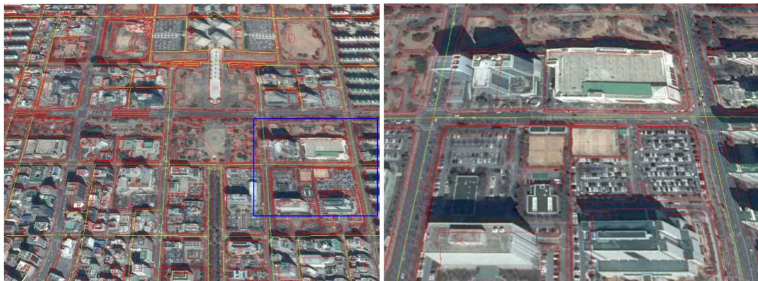
FIGURE 5. Overlap of the OSM(yellow line) and the digital map(red line) in Daejeon
