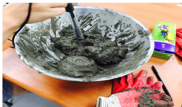
Fig 5. Chloride test Experiment
