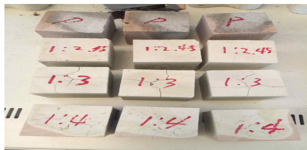
fig 8. Fire resistance test specimens
