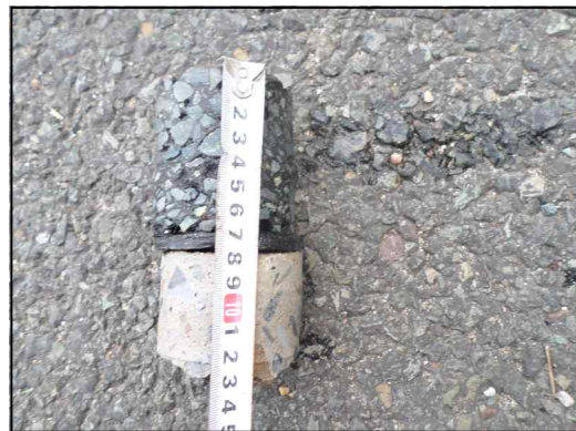
Fig. 3 Measurement of the thickness of the cloth after core sampling
