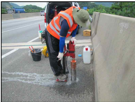
Fig. 2 Core samples of the highway upper surface
