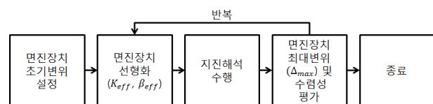
Fig. 2. Flow chart of iterative seismic analysis using equivalent linear model
