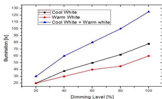
Fig. 8. The illumination measured according to the dimming.
