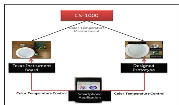
Fig. 9. Test method for measuring the color temperature.
