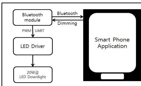
Fig. 1. The proposed LED lighting dimming system configuration.
