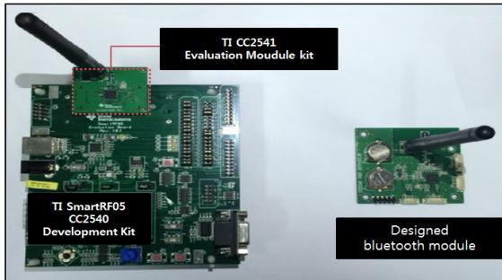
Fig. 4. The implementation of the bluetooth module.
