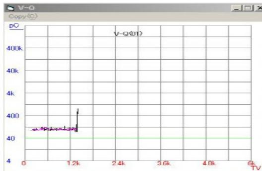
Fig. 4. V-Q properties for non-degraded silicone cable (15 cm+15 cm) contact 2 internal wires.
