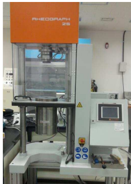
Fig. 2 Capillary rheometer (Göttfert, RG25)
