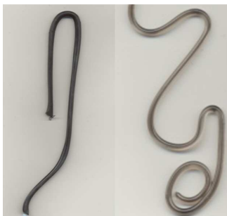
Fig. 5 The extrudates of the PP samples (Left : initial phase, Right : mid-phase)
