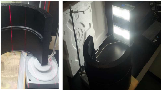
Fig. 8 3D scanning of the thermal butt fusion joint
