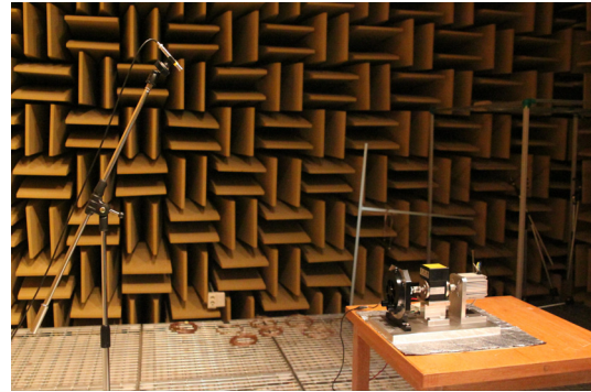
Fig. 5 Noise test in anechoic room
