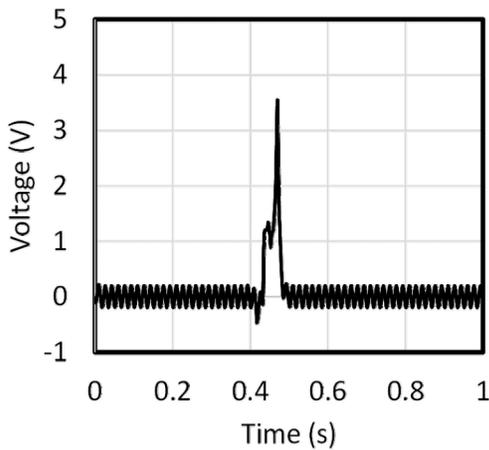
Fig. 3 Output voltage measured with a single droplet
