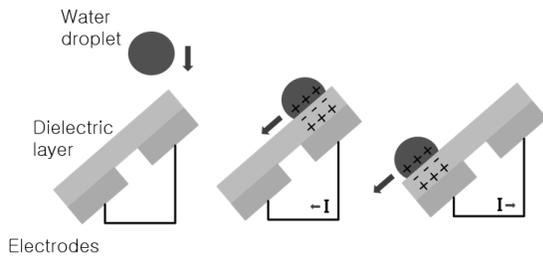
Fig. 1 Working mechanism of REWOD<sup>(2)</sup>
