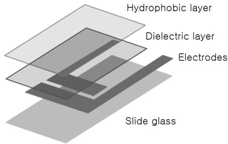
Fig. 2 Schematic of REWOD device
