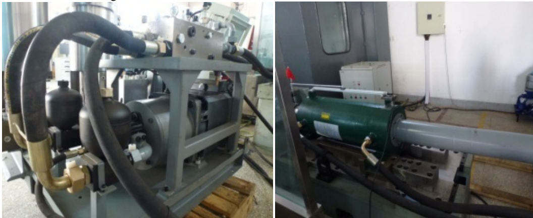
Fig.8 The valve-less electro-hydraulic servo steering device prototype
