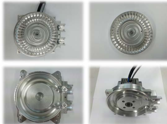
Fig. 7 Manufactured model of newly designed blower
