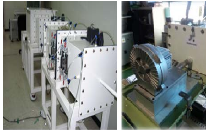
Fig. 11 Performance test facility and blower model
