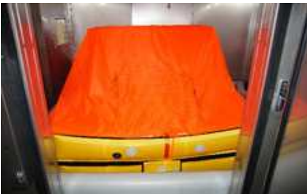
Fig. 4 Life raft in low temperature chamber
