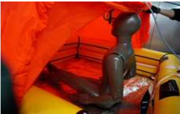
Fig. 3 Experimental condition of thermal insulation assessment using thermal manikin
