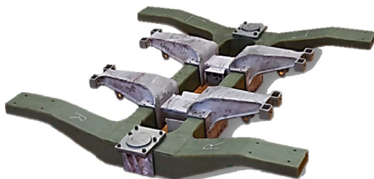
Fig. 1. Bogie structure manufactured by autoclave molding process
