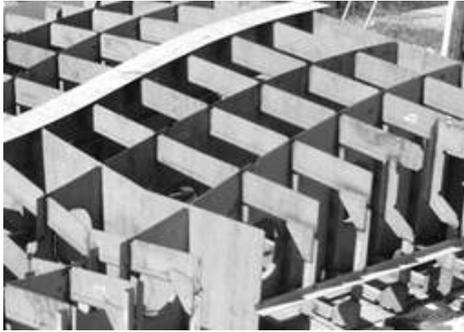
Fig. 2 A Sample welded shell structure
