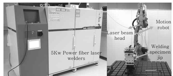
Fig. 1 Experimental setup for fiber laser welding
